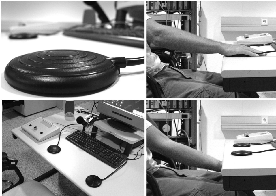
Fig. 2. The participant had to rest his hand on pressure-sensitive sensors (left). When the relevant cue appeared on the screen, he had to press against the top or bottom side of the table (right) with his arm extended.
